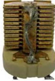
Figure 3.1: The multilayered gold-plated capacitor (geometric capacitance around 71 pF) used for measurements at Roskilde University setup
