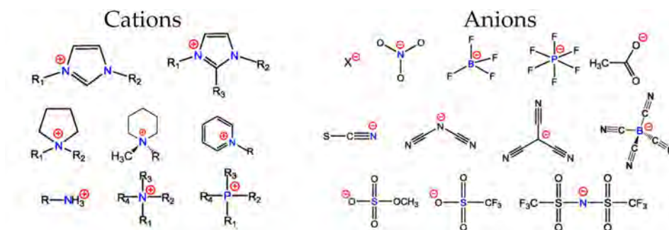
Figure 1.1: Modified version of Fig. 1 from Wang et al. [2020]. Examples of chemical structures of typical cations and anions for ILs.
