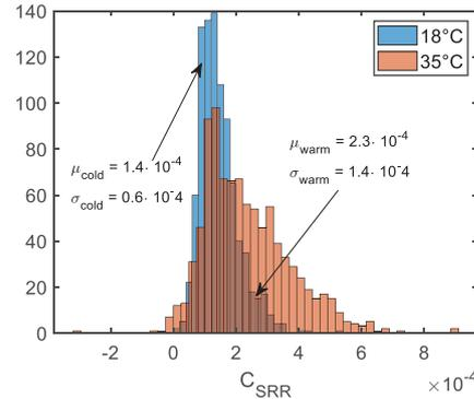
Figure 4. Histogram of measured structural rolling resistance coefficients for cold (18°C) and warm (35°C) road conditions. We see an increase in the mean ( $\mu$ )  $C_{SRR}$  value, when the road temperature is increased. Furthermore, the distribution of measured values is broader under warm conditions (increased  $\sigma$ ).
