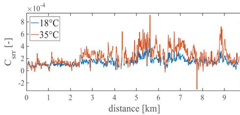
Figure 3. Calculated  $C_{SRR}$  at warm (35°C) and cold (18°C) road temperature. The median of the standard deviations are  $0.13 \cdot 10^{-4}$  (9%) for 18°C and  $0.2 \cdot 10^{-4}$  (5.5%) for 35°C. Note that the  $C_{SRR}$  values are negative in some points at 35°C, which is unphysical. This behavior is commented on in section 4.2.
