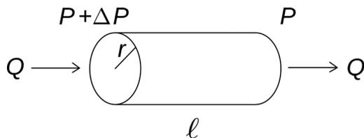
Fig. 2. Fluid flow through a tube due to a pressure difference. Here  $Q$  is the volume of fluid driven through the tube per unit time,  $r$  a characteristic cross sectional width,  $\ell$  the length of the tube, and  $P$  the pressure.
