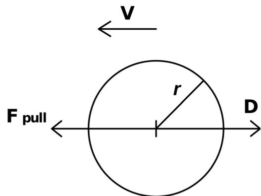
Fig. 1. Drag force on a body pulled through a fluid. Here  $\mathbf{F}_{\text{pull}}$  is the pulling force,  $\mathbf{D}$  the drag force,  $\mathbf{v}$  the velocity of the body, and  $r$  a length characterizing the size of the body.
