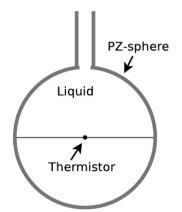
**Fig. 5.** The combined measurement of  $c_l, \kappa_s, \beta_s$ .
