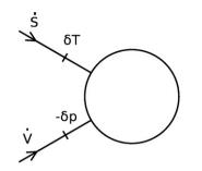
**Fig. 1.** The two scalar energetic interactions with a differential volume element. Differential means that the wavelengths of the thermal and mechanical perturbations are much longer than the dimensions of the volume element.
