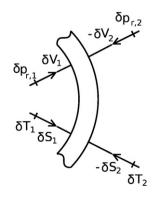
**Fig. 3.** Depiction of the four thermal and mechanical interactions at the boundaries at  $r_1$  and  $r_2$  in spherical geometry.
