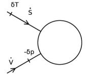
**Fig. 2.** Another response situation. Here entropy and pressure are the input variables and marked on the energy bond nearest to the system. In Fig. (1) temperature and pressure were the input variables.
