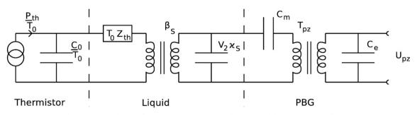
Fig. 6. Equivalent diagram of the liquid in contact with the thermistor and the piezoelectric shell (PBG).
