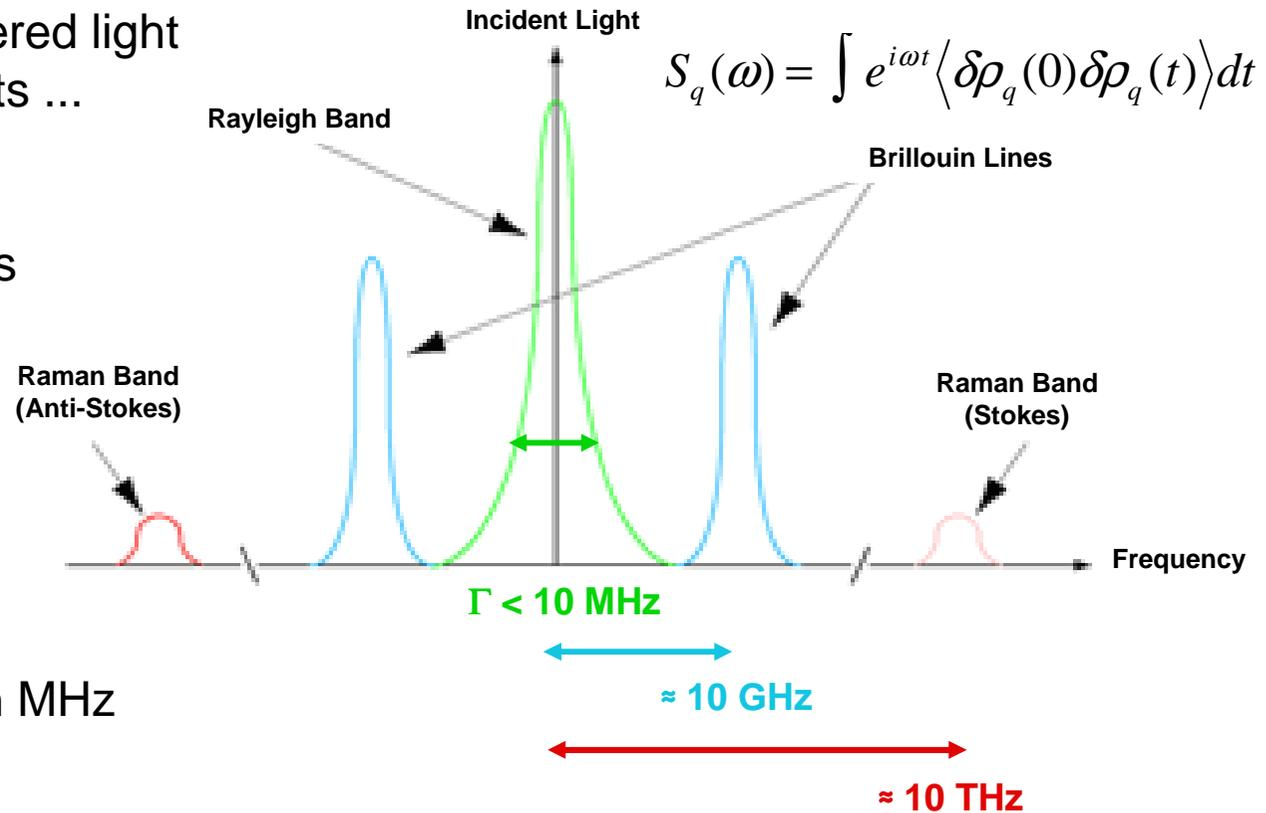
Small energy shifts ( $< \text{MHz}$ ) cannot be measured using filter techniques (grating, Fabry-Perot) but are best resolved in the *time domain* ...
